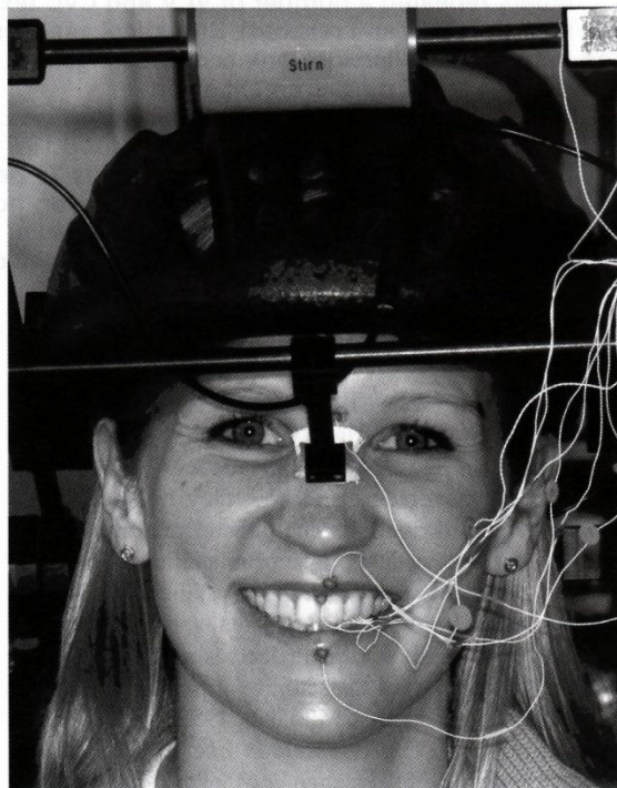
Figure 2 Volunteer with helmet configuration and coils glued in place.
